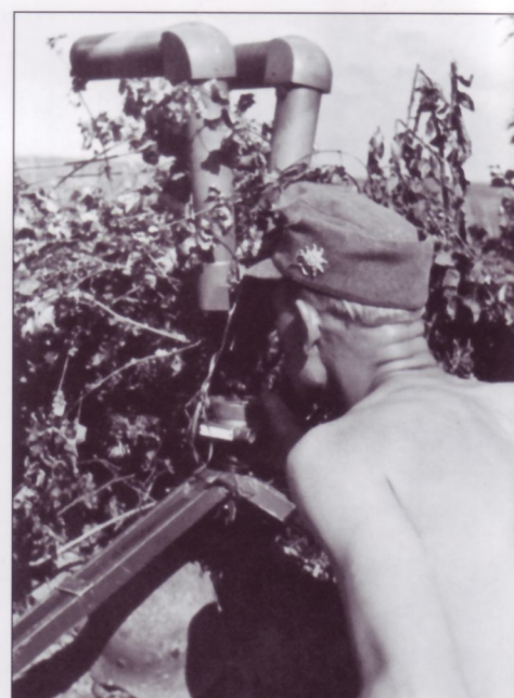
The 6x30 Sf.14Z Scherenfernrohr (scissors binoculars) have been fitted with tube-like sunshade hoods. These served to prevent reflection off the lenses from revealing the forward observer's position and if angled somewhat in the direction of the sun reduced glare. It appears that the sunshades have been camouflage-painted. The instrument itself is normally gray. While the position is well camouflaged, the cut vegetation is wilting and will have to be soon replaced.
