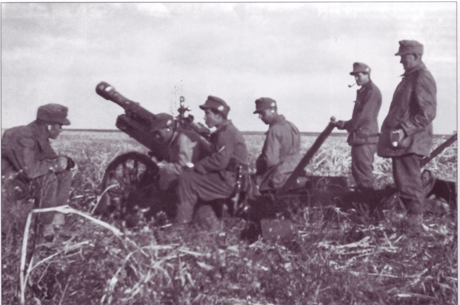
The crew of a Rheinmetall 7.5cm GebG36 Gebirgsgeschütz stands by for orders to fire. This compact weapon was considered heavy in its role as a mountain gun at 750 kilograms (1,654 pounds). It had a range of 9,150 meters (10,010 yards) and a rate of fire of six rounds per minute. These artillerymen wear the silver Jäger cap badge of three oak leaves and an acorn as worn by Jäger-Divisionen (light infantry divisions). An oval cloth version was worn on the upper right arm.
