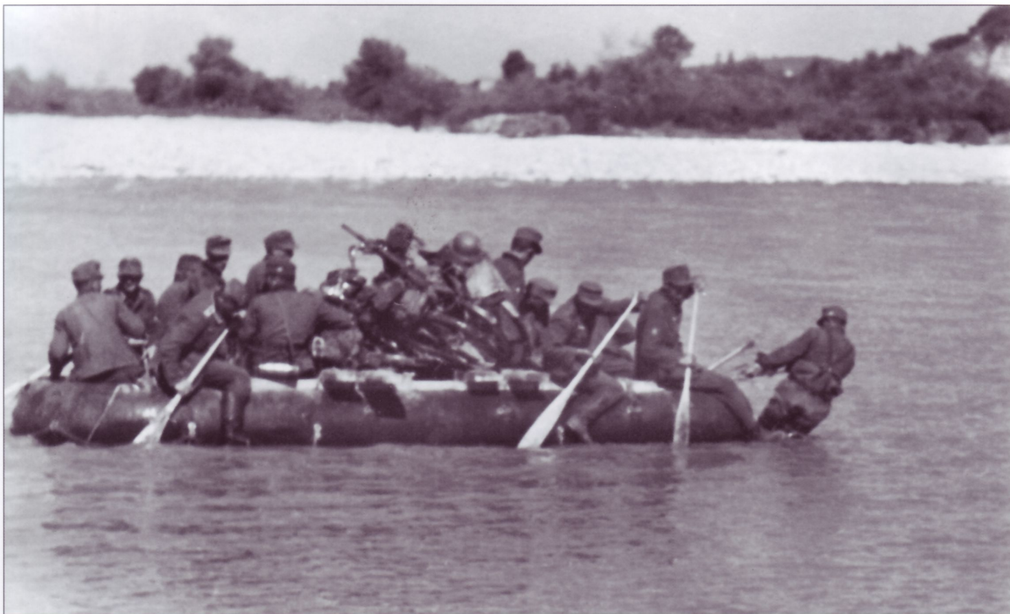
Gebirgsjäger paddle a medium pneumatic boat across a river. These boats were 18 feet in length and had a beam of 6 feet 1 inch. They could carry 1.35 tons of cargo, but were also used to construct pontoon brigades and multi-boat rafts capable of transporting vehicles. Here a number of bicycles are stacked aboard. This river appears to be sufficiently shallow for the boat to have become grounded.
