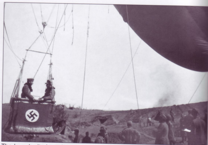
The launch site is on low ground protected by a ridge to limit the effects of artillery fire and for protection from ground winds. Two men went aloft with the balloon: the observer and another to record data and relay it to the ground by telephone. He would also be on lookout for the approach of any aircraft. The crew would be as nervous of approaching friendly aircraft as enemy.
