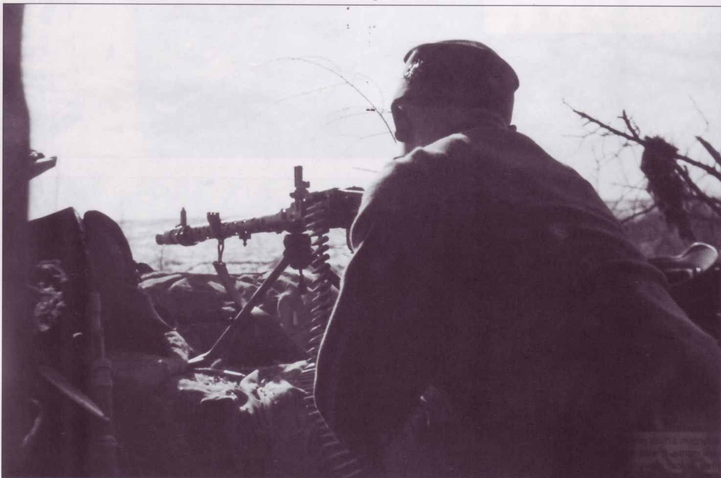
An MG34 machine gun with the bipod fitted rearward for use in a defensive position. German machine gun bunker firing ports were usually much smaller, both in width and height, to make them more difficult to detect and hit.
