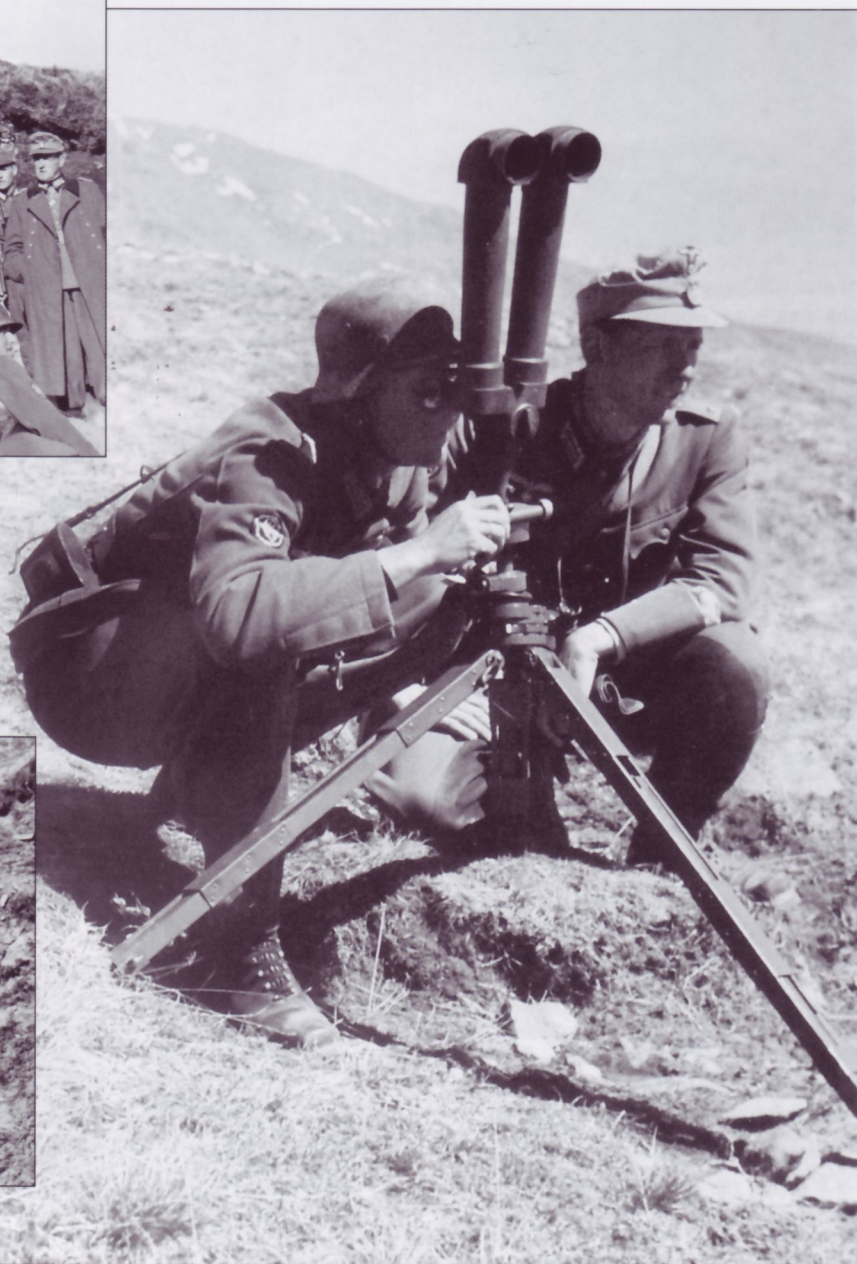
The tripod-mounted 6x30 Sf.14Z Scherenfernrohr (scissors binoculars) was known as the Eselsohren (donkey ears) for obvious reasons. In the U.S. Army this was called a battery commander's or BC scope.
